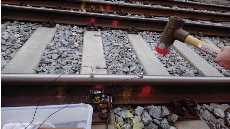
(b) Impact test performed at the additional section close to accelerometer A11.
