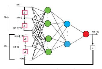
Fig. 1. NARX recurrent neural network architecture
