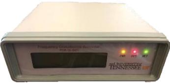
Figure 1. Frequency disturbance recorder (FDR).
