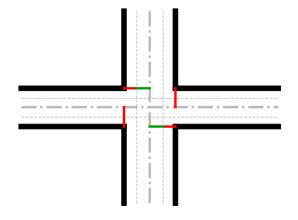
Figure 4: A single four-way intersection with two lanes per direction. Red bars indicate that the corresponding lane is given the red light and stopped, while green bars indicate that vehicles in that lane are allowed to pass. In this particular configuration, the North and South left-turning lanes are given the green light.
