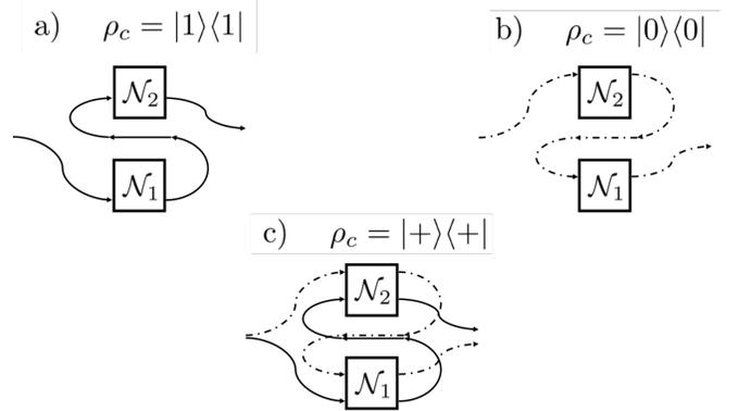
FIG. 1. (a) and (b) illustrate channels  $\mathcal{N}_1$  and  $\mathcal{N}_2$  placed in a definite order, corresponding to the control qubit being in state  $|1\rangle\langle 1|$  and  $|0\rangle\langle 0|$  respectively. In (c) the quantum SWITCH places the channels in a superposition of causal orders. It entangles the order of the two channels with the state of the control qubit, in this case  $|+\rangle\langle +|$ . (c.f. equations 1,2)
