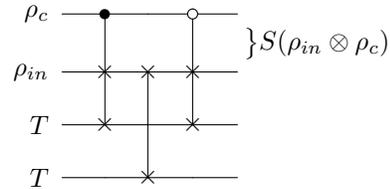
The (controlled) swap gates can be decomposed into toffoli and C-NOT gates. The circuit is then transpiled using the native IBMq transpiler for the allowed operations and connectivity of the particular backend which has been selected for the experiment. The depth of the final transpiled circuit is 31. The circuit consists of 51 gates, of which 19 are two qubit gates. These two qubit gates have a lower fidelity, so care is taken to minimize the number of such gates in the circuit.
