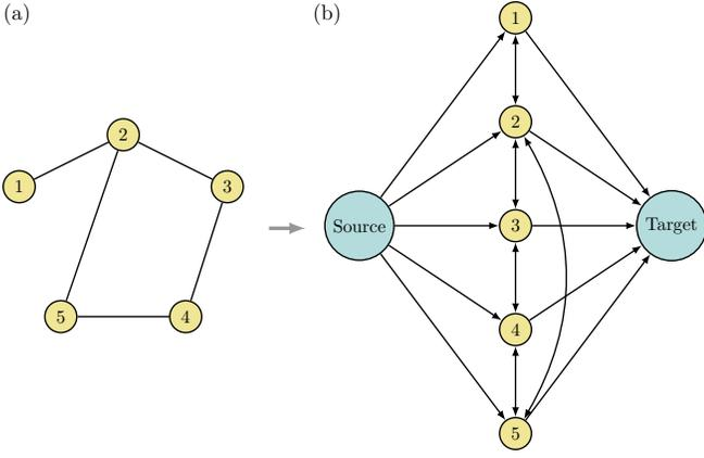
FIG. 8. Mapping the Wasserstein distance defined based on topology to a minimum cost flow problem. (a) Topology  $\mathcal{G}(V, E)$  with 5 vertices and 5 edges, from which the Wasserstein distance is defined. (b) Directed graph of the minimum cost flow problem, which is constructed using the given topology  $\mathcal{G}$ . The minimum cost of the flow problem is equal to the Wasserstein distance.
