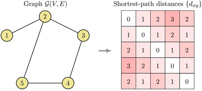
FIG. 3. Example of the Wasserstein distance defined based on a graph consisting of 5 vertices and 5 edges. Given the topology  $\mathcal{G}(V, E)$ , the shortest-path distances  $\{d_{xy}\}$  can be calculated, from which the Wasserstein distance can be defined.
