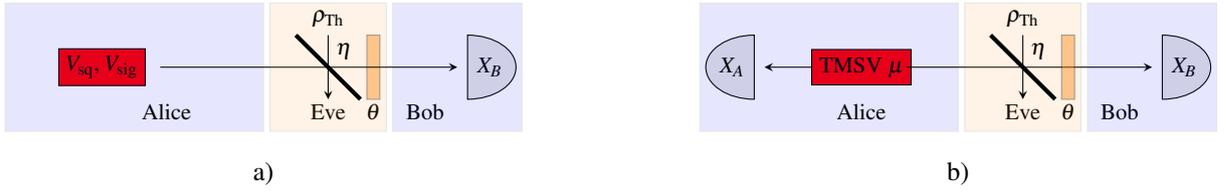
Figure 2: Squeezed-state protocol with homodyne detection in the thermal-loss channel. The phase shifter  $\theta$  represents the phase noise  $\sigma_\theta^2$ . Shown in a) is the equivalent prepare and measure squeezed-state protocol and in b) is the entanglement-based version of the squeezed-state protocol.
