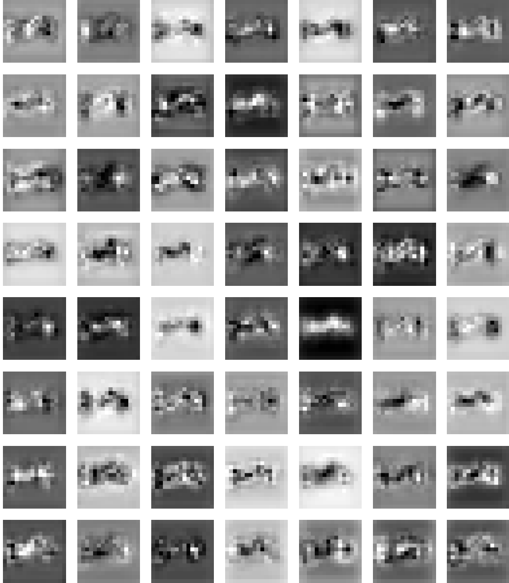
Figure 13: Example of the features enhancement in the third layer. All 56 filters are shown, and each filter tries to detect different enhanced local features of the tracks.
