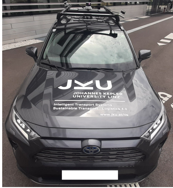
Fig. 3: JKU-ITS Automobile picture showing the LIDAR sensors and cameras mounted over the roof rack
