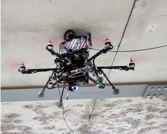
**Fig. 1** Our aerial robot during a layouting mission on a construction site accurately marking points on a concrete ceiling.
