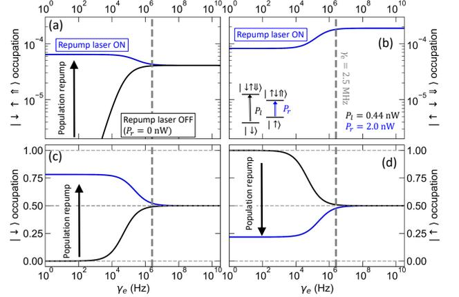
Figure 4. Steady-state trion states (a, b) and electron ground-state spin (c, d) occupation probability as a function of electron spin-flip rate, with (blue) and without (blue) repump laser. The dashed lines show the determined spin-flip rate of  $\gamma_e \approx 2.5$  MHz.
