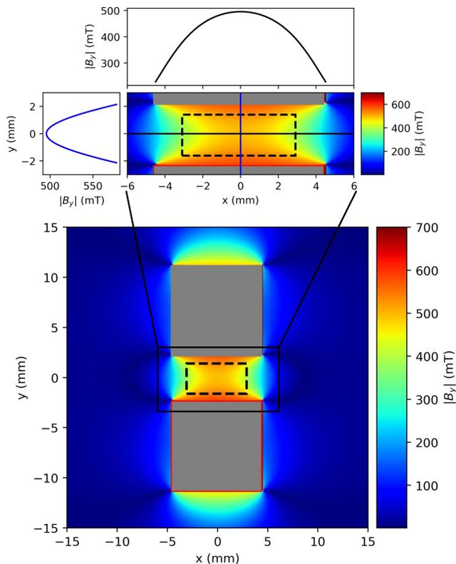
Figure A1. Magnetic field simulation of the magnetic assembly with a 4.5 mm air gap at room temperature. The magnitude of the magnetic field strength  $|B_y|$  along an  $xy$ -cross-section of the assembly (grey regions), with the location of the sample taken to be the origin (outlined by the dashed line). (Inset) Zoom-in  $|B_y|$  to the sample region with cross-sections along the  $x$  (top) and  $y$  (left) direction through the center of the sample.
