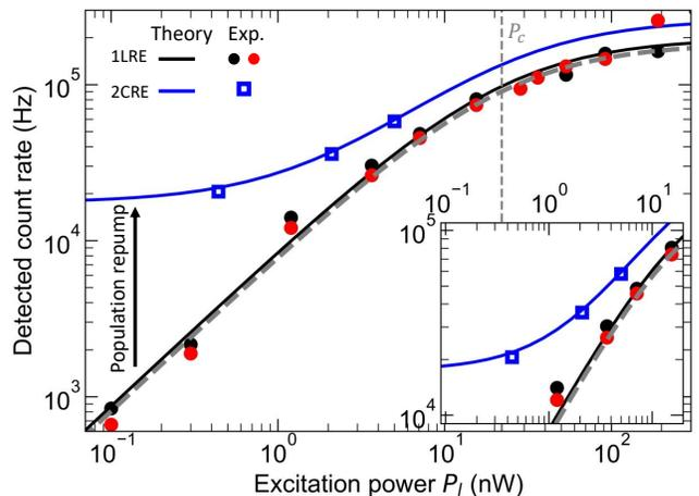
Figure 5. Power dependency of the trion resonant fluorescence under different excitation schemes, comparing experimental photon count rates (symbols) to our model (lines) with  $\gamma_e = 2.5$  MHz: Only pump laser for both trion transition (1LRE, black and red) and with repump laser (2CRE, blue). The gray dashed lines indicate the standard two-level system saturation behaviour.
