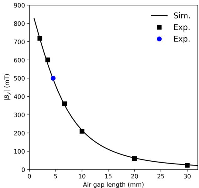
Figure A2. Air gap length dependence of magnetic field strength  $|B_y|$ . The experimental Hall probe data points taken before (black) and after (blue) fixing SmCo magnets into copper mount are compared to at the sample center simulated  $|B_y|$  (curve).
