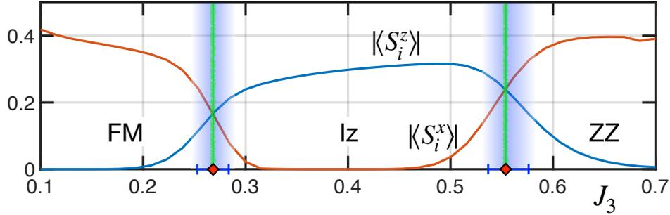
FIG. S1.  $|\langle S_i^z \rangle|$  and  $|\langle S_i^x \rangle|$  along the length of a  $16 \times 40$  cylinder in a DMRG scan vs  $J_3$  for the  $\Delta=0$  limit of the  $J_1^\Delta$ - $J_3$  model. The crossing points are the phase boundaries and the shaded regions are the error bars.
