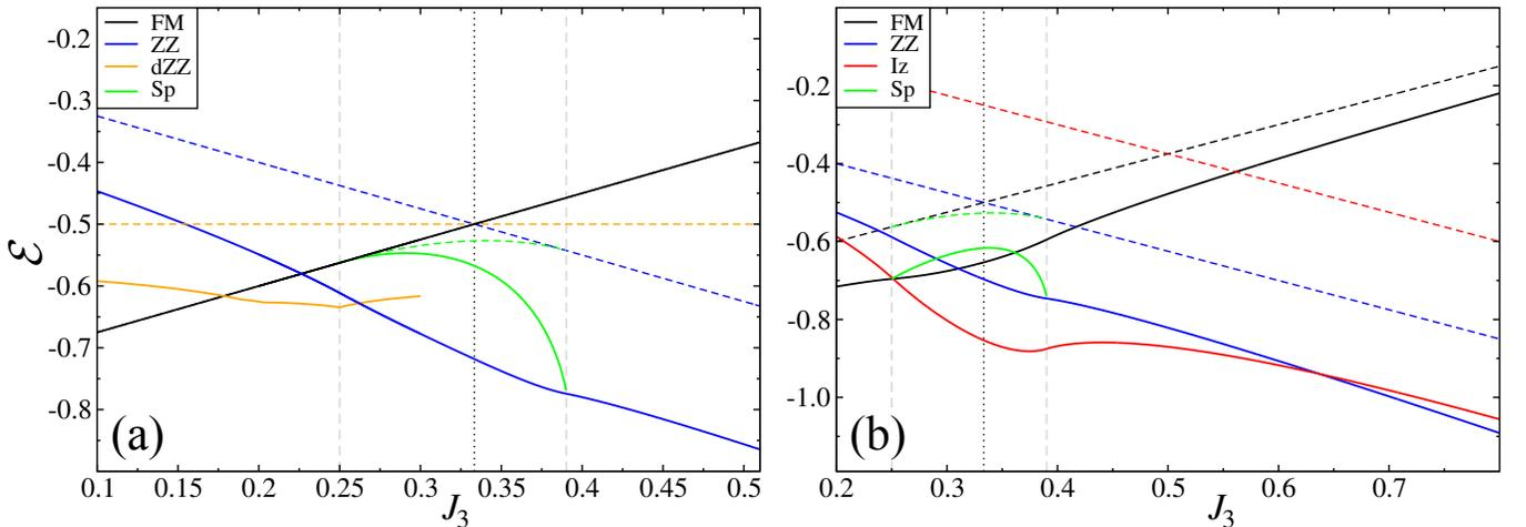
FIG. S8. (a) The classical (dashed lines) and quantum (solid lines, from (2)) energies of the FM, ZZ, Sp, and dZZ states vs  $J_3$  for  $\Delta_{1(3)}=1$  per atomic unit cell. The vertical dashed lines are classical FM-Sp and Sp-ZZ boundaries and the dotted line is the crossing of  $E_{cl}$  for the FM and ZZ states. (b) Same as (a) for the FM, ZZ, Sp, and Iz states for  $\Delta_1=0$  and  $\Delta_3=1$ .
