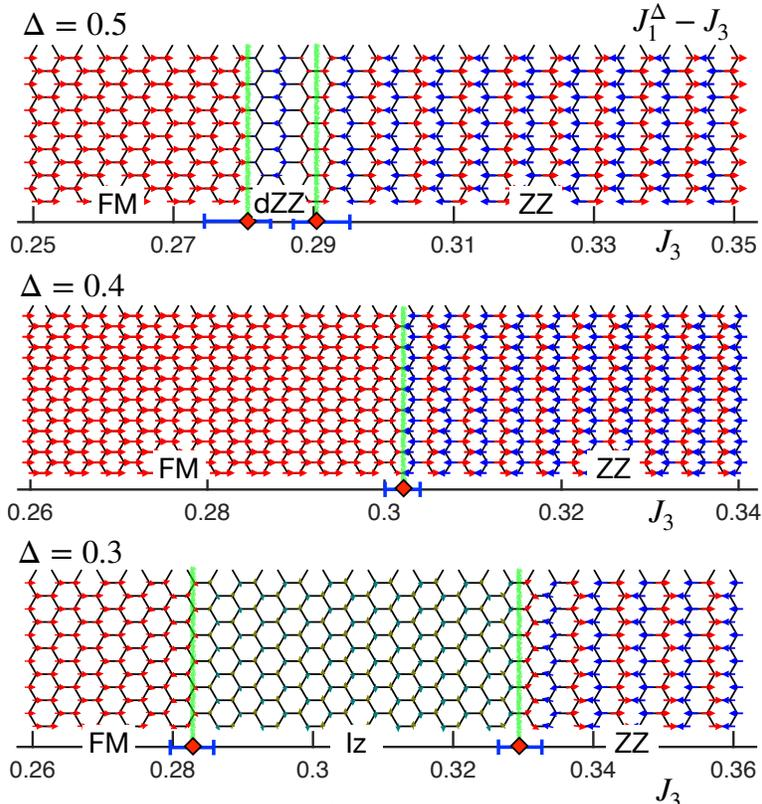
FIG. S3. DMRG  $J_3$ -scans for  $\Delta=0.5, 0.4,$  and  $0.3$  in the  $J_1^\Delta - J_3$  model. The scans for  $\Delta=0.5$  and  $0.3$  are on the  $12 \times 32$  cylinders while the  $\Delta=0.4$  scan is on the  $16 \times 40$  cylinder.
