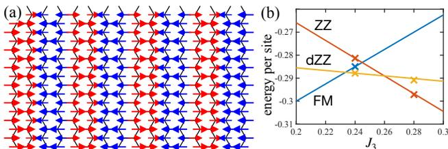
FIG. 3. (a) Ordered moments in the  $16 \times 16$  non-scan cluster for  $J_3=0.24$ , showing dZZ pattern. (b) Energies of the three competing phases vs  $J_3$ , crosses are DMRG results and higher-energy states are metastable. Lines are extrapolated energies,  $\langle \psi_i | H(J_3) | \psi_i \rangle$ , where  $\psi_i$  are the three states at  $J_3=0.24$ .
