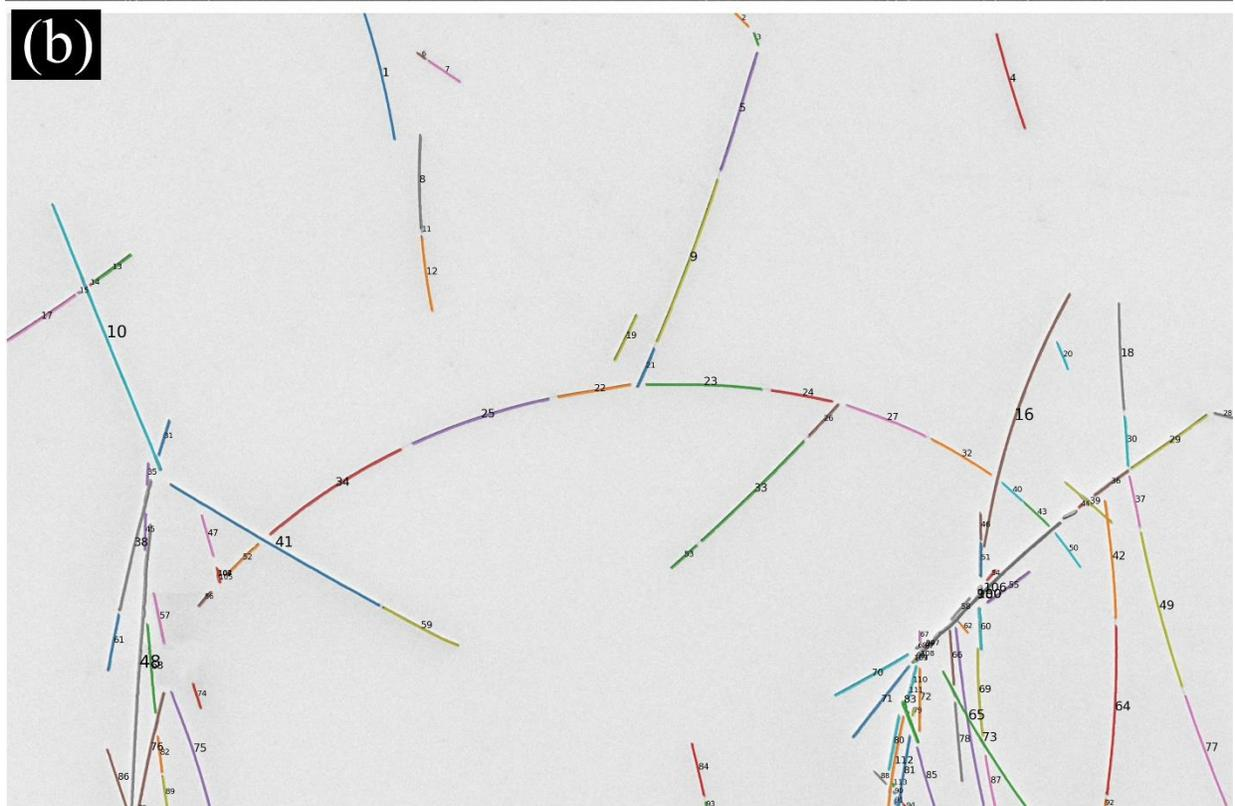
Figure 4. (a) Ag nanowires fragmented by thermal annealing and (b) their analyzed image.
