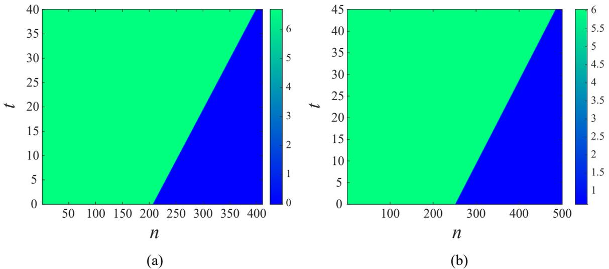
Figure 13: Space-time strain evolution initiated by computed superkink solutions with velocities (a)  $V = 4.8$ ; (b)  $V = 5.2$ . Here  $a = -1$ ,  $b = 10$ .
