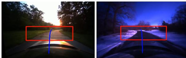
Figure 9. Lane-Keeping task. Red rectangle indicates the input and blue line shows the predicted steering angle of the network. Left is shown summer condition, and right is shown winter condition.
