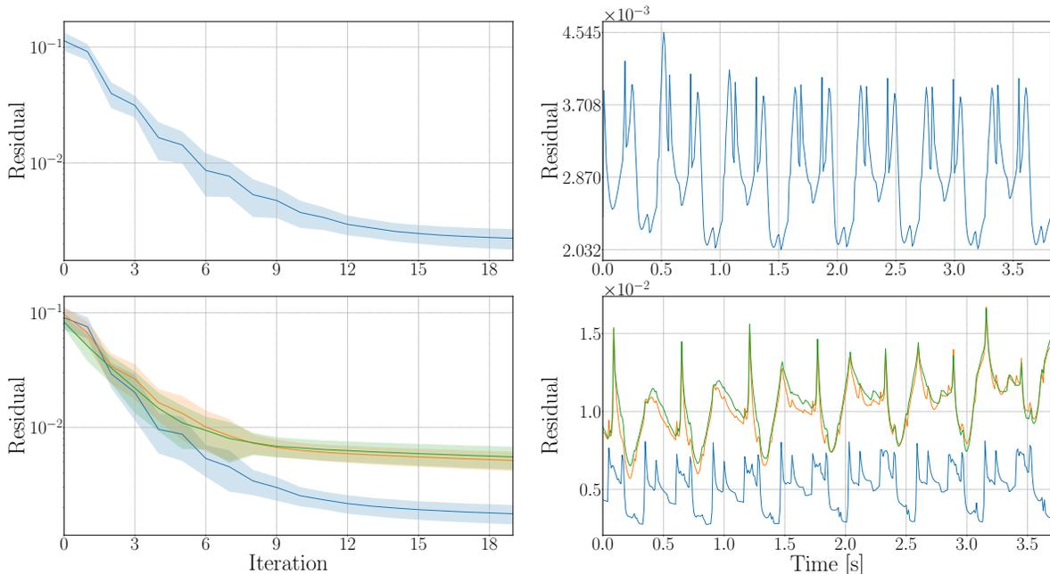
Fig. 4. The two plots on the left show the trend of the  $l_2$  norm of the residuals along the iteration of Algorithm 1. On top is the residual for the quadruped with no arm, while on the bottom are the residuals for the quadruped manipulator. The right side plots show the time plot of the residual norm while the robot is trotting in simulation. Again, the top plot is for the robot with no arm, and the bottom one is for the quadruped manipulator.
