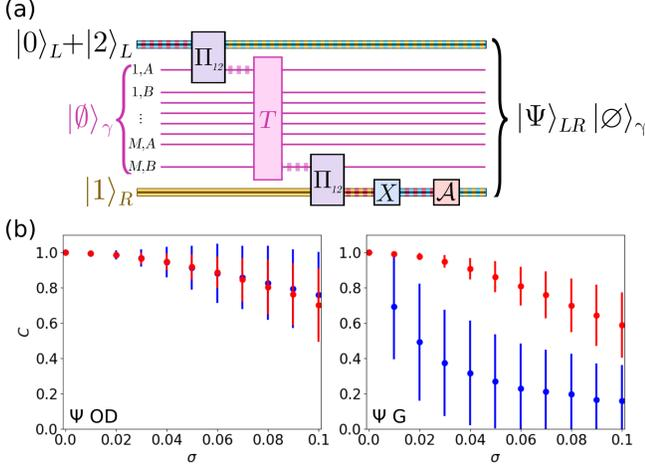
Figure 10. (a) GHZ-like protocol, adapted to create state  $|\Psi\rangle$ . States 0,1 and 2 are shown in blue, yellow and red, respectively. A photon in a cavity is shown as purple shading. (b) Concurrence as a function of disorder strength for off-diagonal disorder (left) and general disorder (right) for an SSH chain with one domain and 14 sites (blue), and for a four-domain chain with 15 sites (red).
