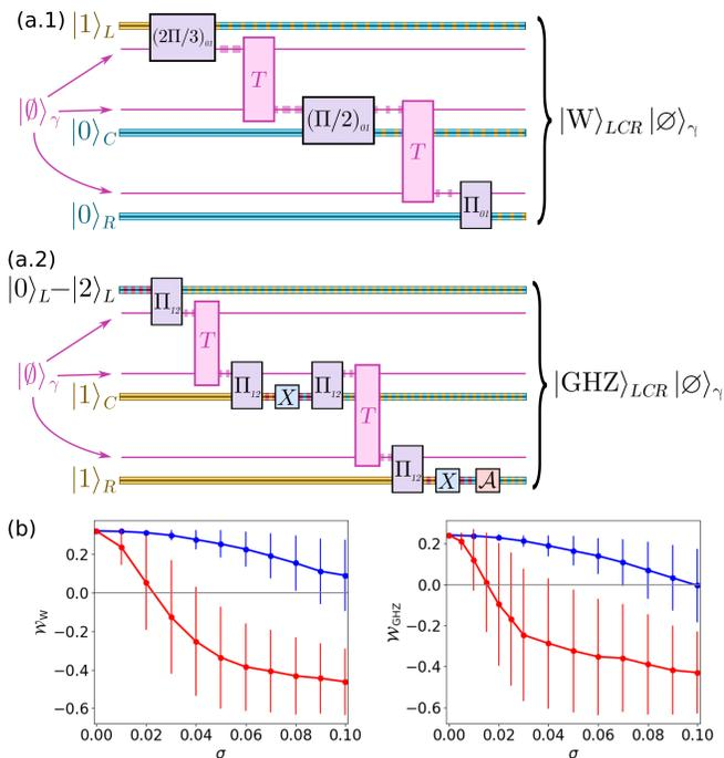
Figure 4. (a) Preparation protocols for (a.1) W and (a.2) GHZ states for 3 qudits:  $L, C, R$ . Qudit states are represented as blue (0), yellow (1) or red (2). Photonic cavities are represented as thin pink lines, with an additional shading if a photon is present. Superpositions are represented with dotted lines. (b) Average values over 1000 realizations of the witnesses in Eq. 12 and Eq. 13 as a function of off-diagonal (blue) and general (red) disorder.
