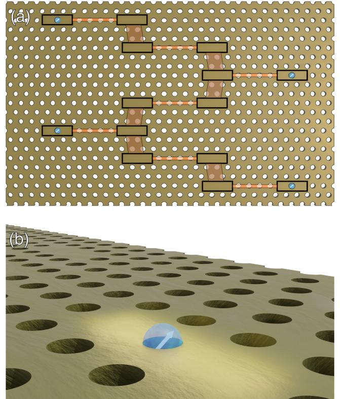
Figure 1. (a) A three-domain, 14-cavity Si photonic lattice. The four color center qubits are represented as blue spheres. (b) Close-up of a color center qubit in a cavity (highlighted).
