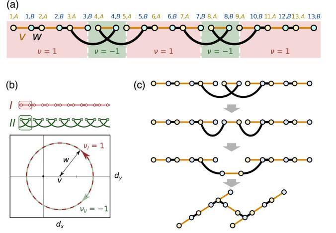
Figure 7. (a) Possible 1D indexing of the cavities, that allows the domains to be identified as having a winding number of  $\nu = \pm 1$ . (b) Path taken in the space of possible Hamiltonians  $\mathcal{H}(k) = \vec{d} \cdot \vec{\sigma}$ , where  $\vec{\sigma}$  are the Pauli matrices and  $k \in BZ$ , for systems I and II above. (c) Under deformation, the lattice in (a) is equivalent to a three-domain lattice of the type shown in Fig. 2 (a).
