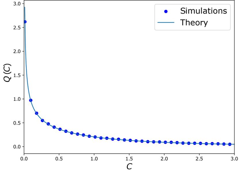
FIG. 3. Distribution  $Q(C)$  of the cost  $C$  until first return for jump distribution  $f(\eta) = e^{-\eta^2}/\sqrt{\pi}$  and cost function  $h(\eta) = \eta^2$ . The continuous blue line corresponds to the exact result in Eq. (62) while the dots are obtained from numerical simulations with  $10^6$  samples.
