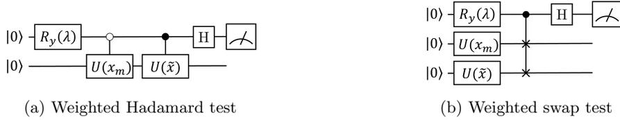
Fig. A.1: Quantum circuit diagrams for (a) weighted Hadamard test (WHT) and (b) weighted swap test (WST), used to implement the QKCs without data superposition. By aggregating the expectation values of the circuit for each training data point, the QKCs can be constructed without data superposition.
