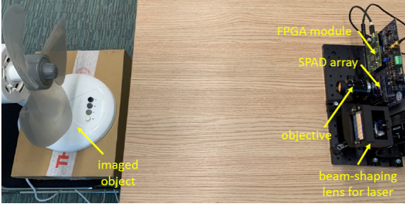
Figure 9. Experimental setup to capture the real SPAD data. The sensor we used here is 192 \times 128 SPAD developed by Henderson et al. [18].
