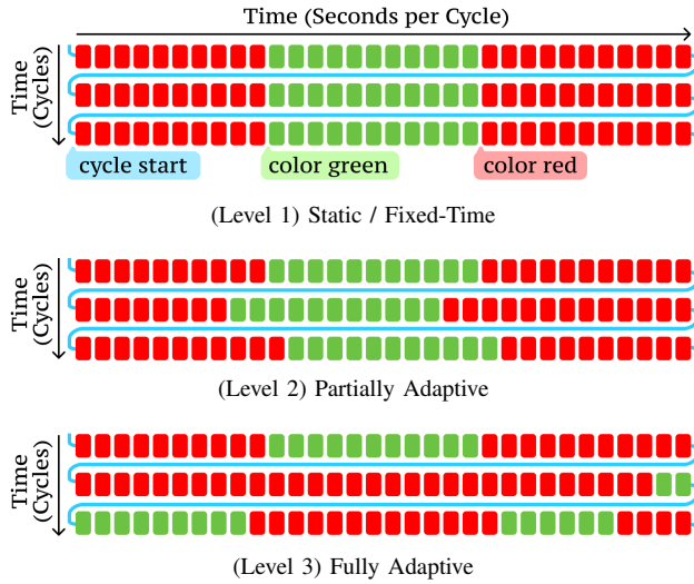
Fig. 1. Possible switching behaviors of traffic lights and the resulting patterns between cycles depending on the short-term adaptivity level.
