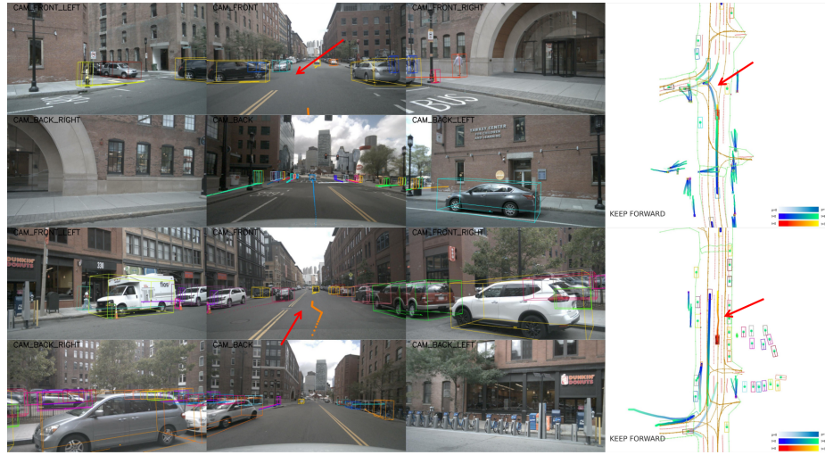
Fig. 4: The qualitative visualization of the planning trajectories. The images from six cameras are shown on the left. The predicted trajectories of traffic agents and the planning result of the ego vehicle are shown on the right. The color intensities of these trajectories vary according to the probability p and the time t . The red arrows highlight the environments which most likely influence the ego vehicle planning.
