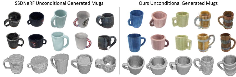
Fig. 8: Qualitative comparison between unconditional generative models training on Objaverse Mugs. We present two renderings and extracted mesh from each generated NeRF. Our approach exhibits a notable advantage in reasonable geometry, particularly for shapes that suffer from self-occlusions when trained only with image supervision.
