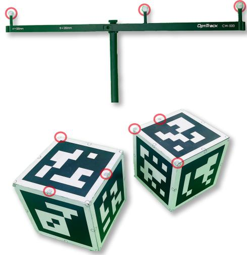
Figure 9. **Illustration of Platform Calibration Tools.** The top is the vender-provided calibration wand for the MoCap system. The bottom are the ArUco cubes attached with reflective markers (circled in red). The ArUco patterns are for unifying the camera in the multi-camera system, while the surface-attached reflective markers are used for unifying the cameras with the MoCap system.
