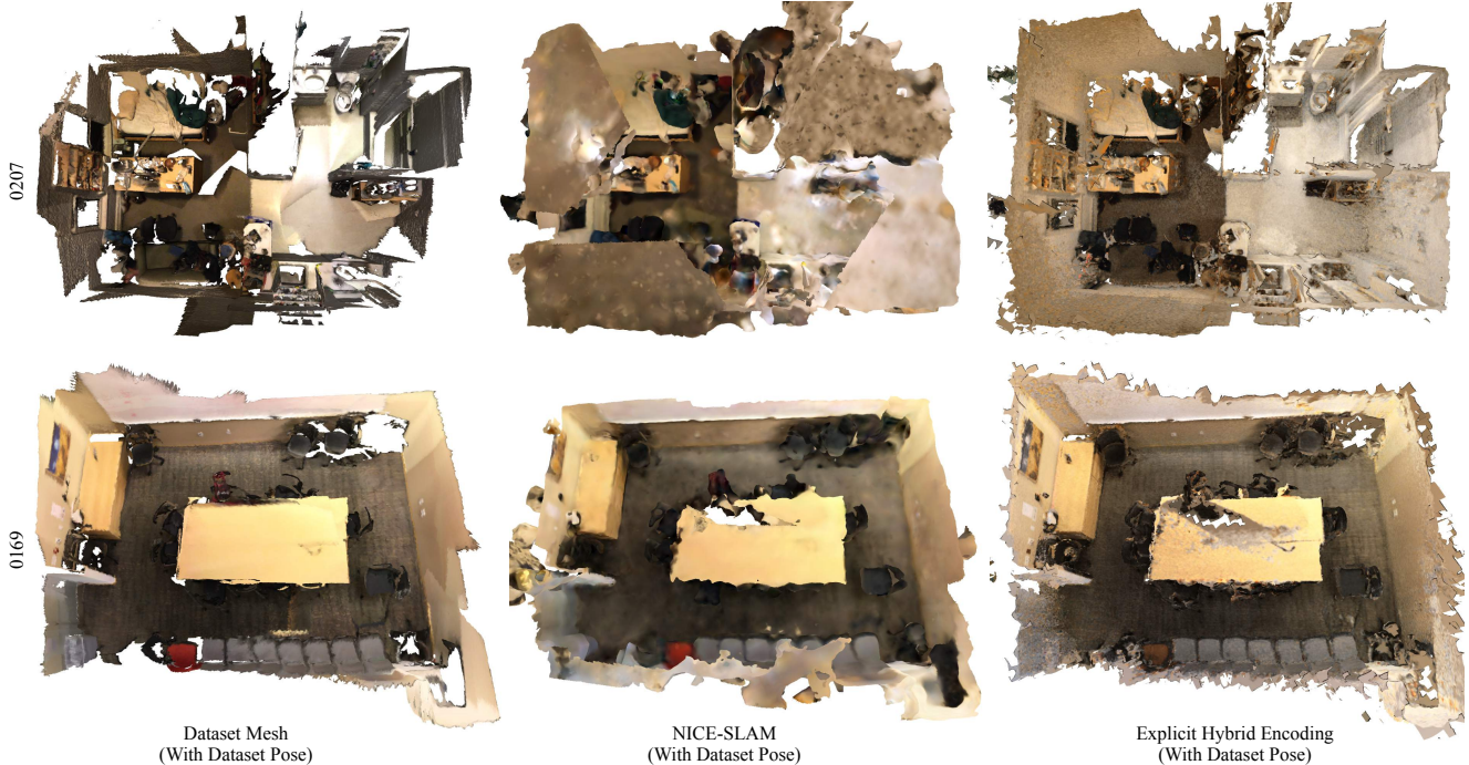
Figure 11. Qualitative evaluation of Hybrid Explicit Encoding on ScanNet Dataset. Both NICE-SLAM and Ours run on the posed RGB-D stream to simulate an externally provided tracker.
