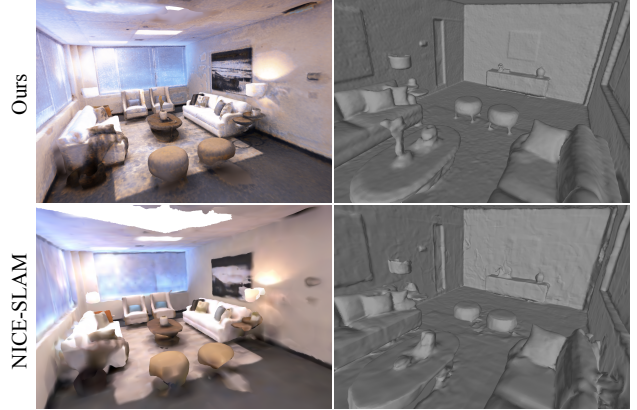
Figure 10. Dense Grid (density) compared to NICE-SLAM under benchmark configurations (Dimensions×Resolutions are 2×2 for Ours vs 32×3 for NICE-SLAM).
