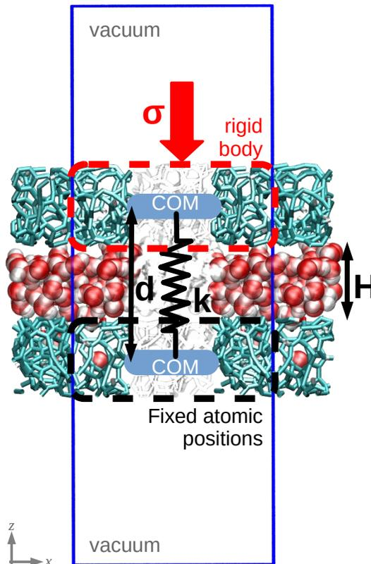
FIG. S9. **Setup of the simulations.** The constructed slit pore is periodic in the  $xy$ -plane and separated by a vacuum layer of 4 nm. A Hookean spring of equilibrium length  $d$  is acting between the center of mass of the two surfaces resulting in the surface separation  $H$ . A stress  $\sigma$  is applied on the fluctuating surface via a homogeneous force density  $f_z$  in  $z$ -direction.
