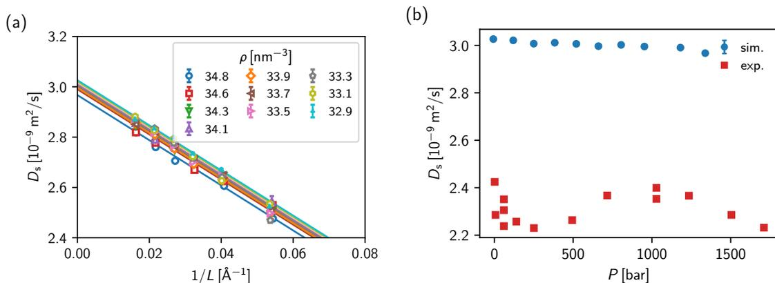
FIG. S11. **Self-diffusion coefficient in bulk water.** (a) Rigorous finite size scaling analysis of  $D_s$  vs. the inverse cubic box size  $L$ . (b) Extracted self-diffusion coefficient  $D_s$  at infinite system size as a function of the pressure  $P$  in the liquid phase. Simulations denote results from this work extracted in (a), experimental data are taken from Krynicki et al.[10]
