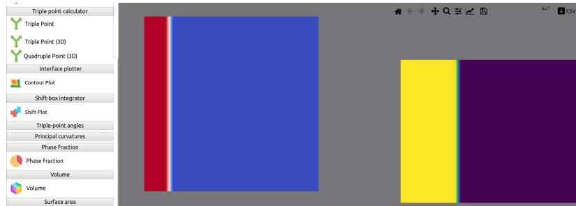
Fig. 45. Illustration of the usage of "Shiftplot" that integrates simulation results into one single frame such that the entire microstructural evolution history may be accessed.
