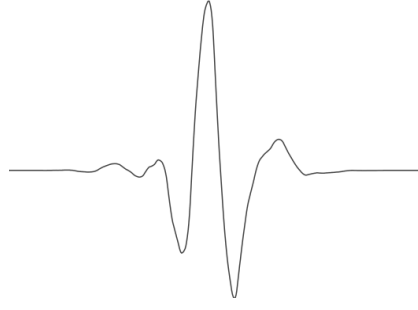
Figure 6: Typical shape of sym5 wavelet used to decompose the ECG signals
