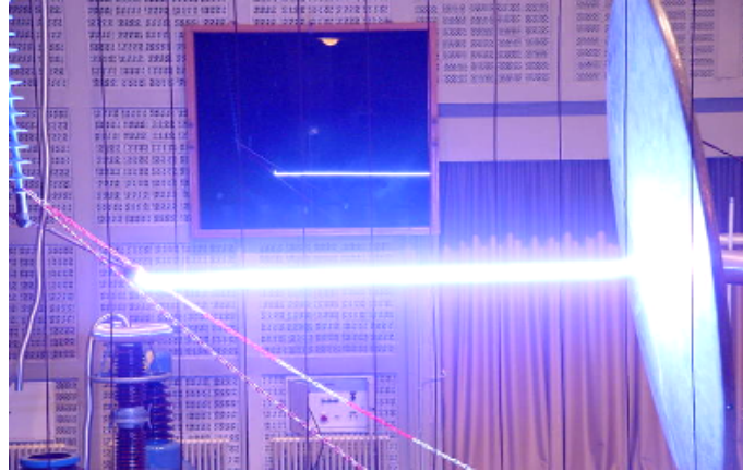
Figure 3: Picture of a laser-guided negative discharge. Adapted with permission from [Rodriguez2002] © Optical Society of America
