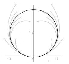
On the left, we have plotted some geodesics for  $\hat{g}$  with  $\alpha = 42$  (their projections for the center of mass (x, y)). The black circle through the origin is the nonholonomic trajectory through the origin with initial velocity
