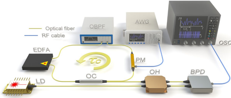
Fig. 1. Photonic architecture for generating microwave waveforms with programmable chirp shapes. A phase-modulated optical fiber loop (round-trip time: \tau_c ) comprising an electro-optic phase modulator (PM), an optical bandpass filter (OBPF), an erbium-doped fiber amplifier (EDFA), and an optical coupler (OC), is utilized as an optical oscillator. A chirped optical waveform with a chirp shape identical to the low-frequency driving waveform from an AWG will be produced from the phase-modulated optical fiber loop. The output chirped optical signal is then down-converted to microwave domain by using an optical coherent detection device containing a 90° optical hybrid (OH) and a balanced photodetector (BPD), where a narrow-linewidth single-frequency laser from a laser diode (LD) acts as a local oscillator signal. The generated chirped microwave waveform is recorded by using an oscilloscope (OSC).
