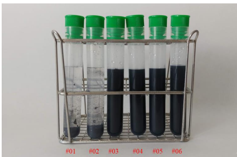
Figure 2. 5 Photograph of the milled wet ball-milling GO synthesis test samples in water solution after 24h.
