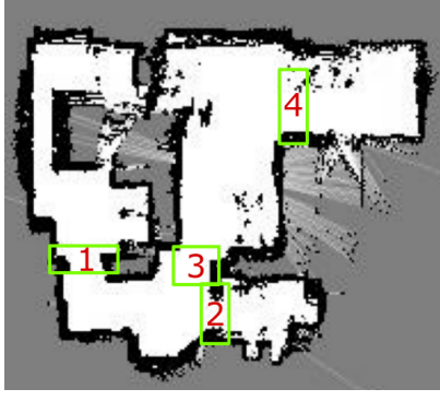
Fig. 7. Door detection results marked on an LiDAR based occupancy grid map
