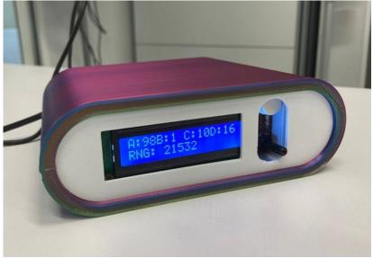
Figure 9: pRNG prototype.
