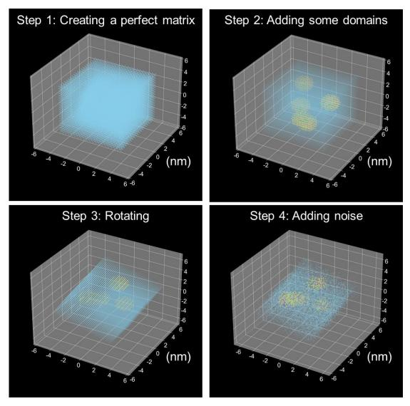
**Fig. 2** Pipeline of simulated APT data. Adding some specific nano-structures  $(Al_{0.75}Li_{0.2}Mg_{0.05}$  nanoparticles here) into a perfect FCC matrix, then rotating and disturbing to simulate the crystallographic orientation and trajectory abbreviation encountered in APT data, respectively.
