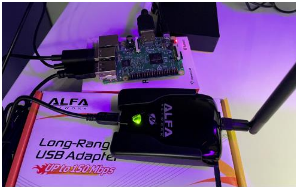
Figure 17: Alpha Wi-Fi adaptor and Raspberry- Pi 3 (Primary Source).
