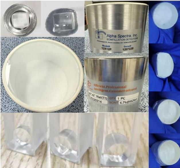
**Fig. 1.** NaI:Tl samples with different sizes and shapes.
