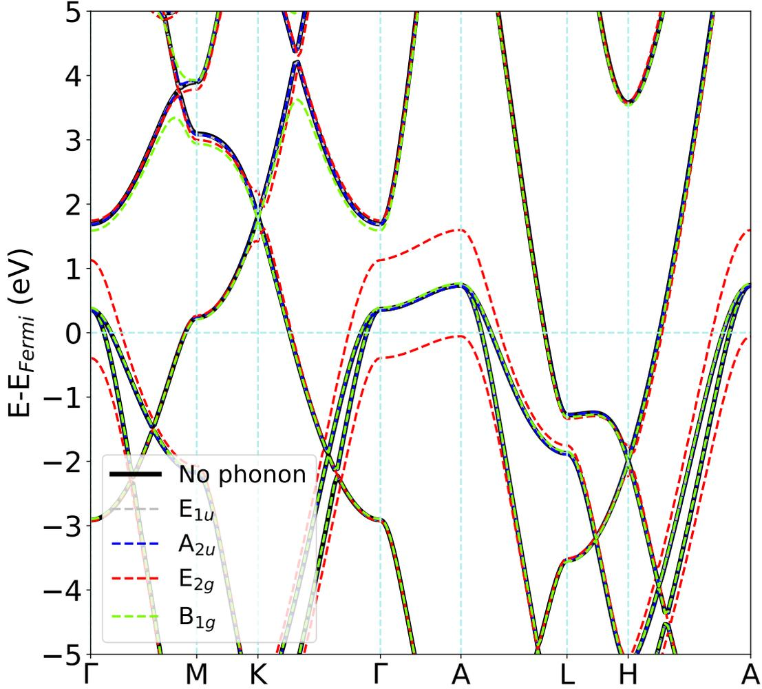
FIG. 3. Electronic band diagrams of the  $\Gamma$  frozen phonons in  $\text{MgB}_2$  compared to the band structure of the unperturbed system. It becomes clear that only the  $E_{2g}$  phonon strongly perturbs the electronic bands near the Fermi energy and so will be the only band that contributes to the EPC.
