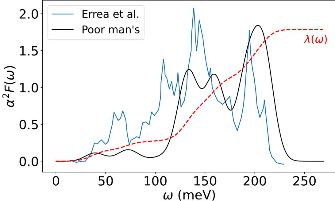
FIG. 6. The  $\alpha^2 F(\omega)$  function approximated from the poor man's approach for  $\text{H}_3\text{S}$  at 200 GPa using a  $2 \times 2 \times 2$   $q$ -mesh compared to that reported by Errea et al. [24] where a  $6 \times 6 \times 6$   $q$ -mesh was used. The red dashed line shows  $\lambda(\omega)$  calculated from  $\alpha^2 F(\omega)$ .
