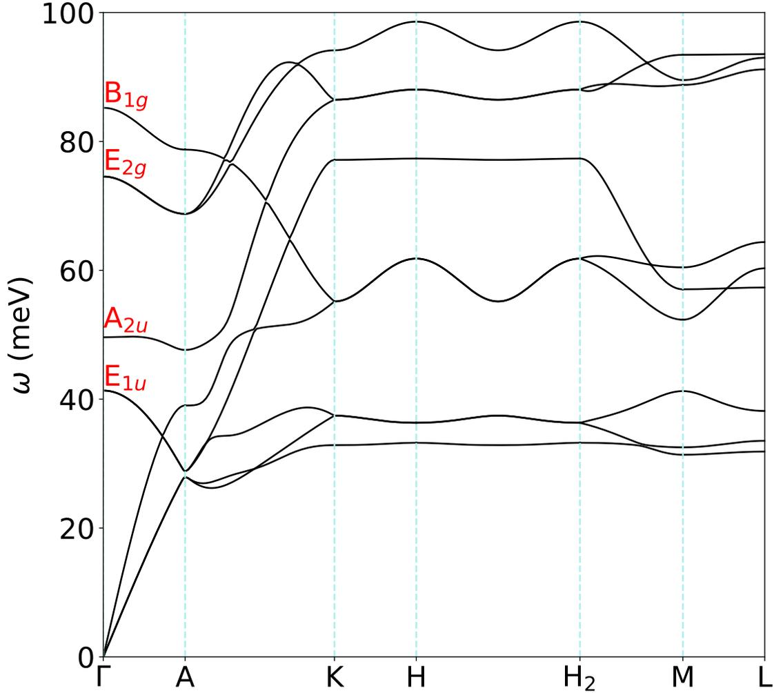
FIG. 2. Phonon band diagram of MgB<sub>2</sub> with the  $\Gamma$ -modes labelled.
