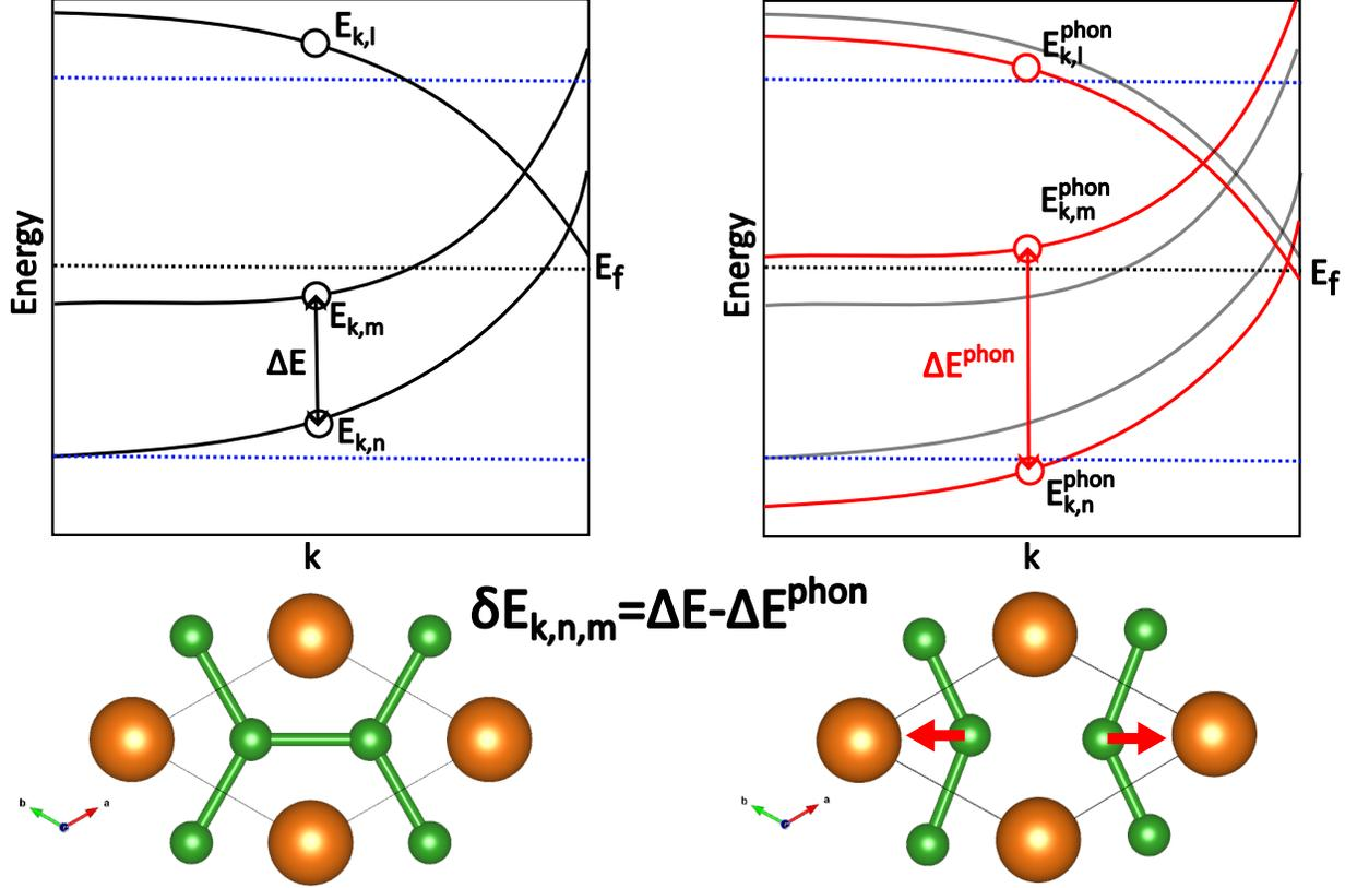
FIG. 1. Explanatory diagram showing how  $\partial E_{k,n,m,q,\nu}$  is calculated from the difference in electron energy band splittings for a phonon described by wave vector  $q$  and band  $\nu$ . The blue dashed line indicates the energy window corresponding to the maximum phonon energy of that system.
