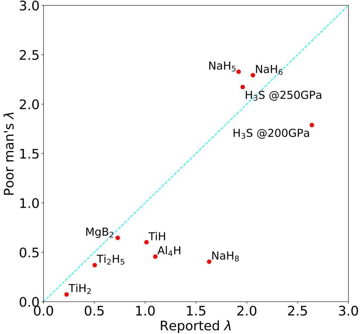
FIG. 4. A scatter plot of  $\lambda$  calculated using the approximation described in this paper and a Gaussian width of 0.06 Ry (81.6 meV) against that reported in the literature [1, 2, 20, 24, 25].
