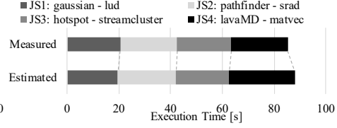
Fig. 8. Comparison of Measured vs Estimated Time ( JobMix3, P_{total} = 400[W] )
