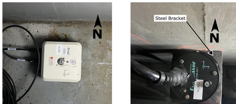
Figure 2.2: Fastening of accelerometers at the bottom (left) and mid-height (right) of the reaction mass
